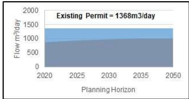
Figure 3: Recorded and predicted dry weather flow with existing permit
