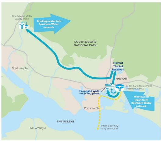
Figure 1-1 - Transfer from Budds Farm WTW to Otterbourne WSW via WRP and HTR
