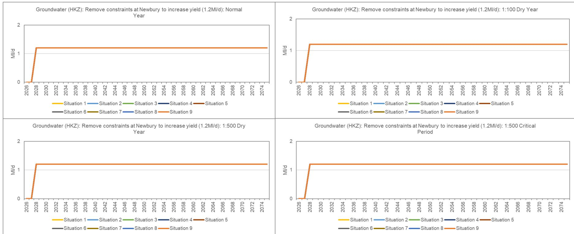
Figure 15: Utilisation of Newbury groundwater source in HKZ in each supply-demand situation under each planning scenario.
