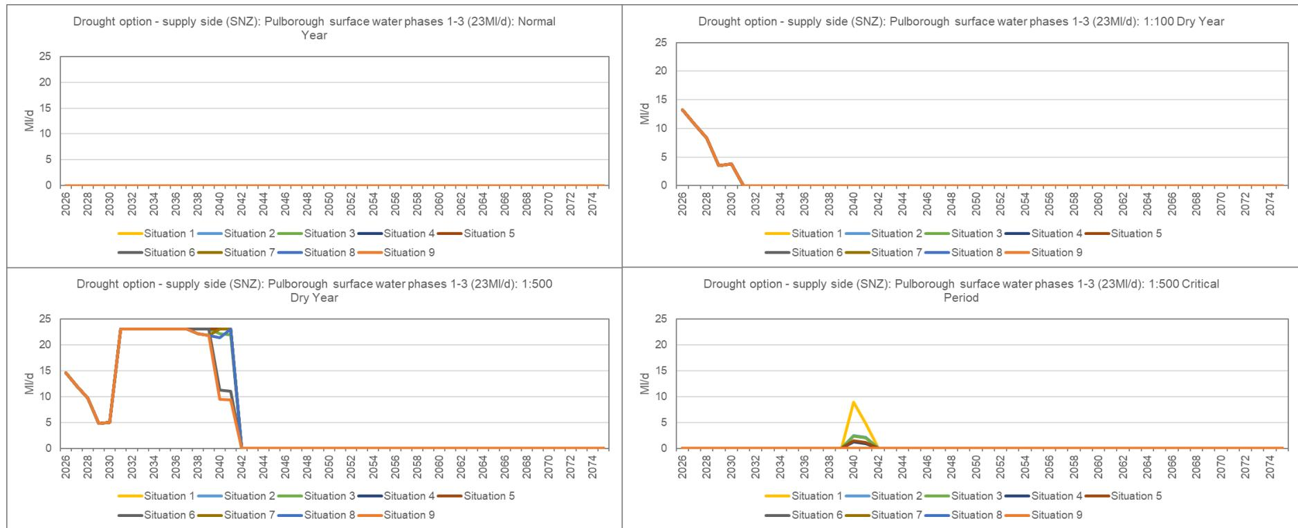
Figure 34: Utilisation of Pulborough surface water drought option in SWZ in each supply-demand situation under each planning scenario.
