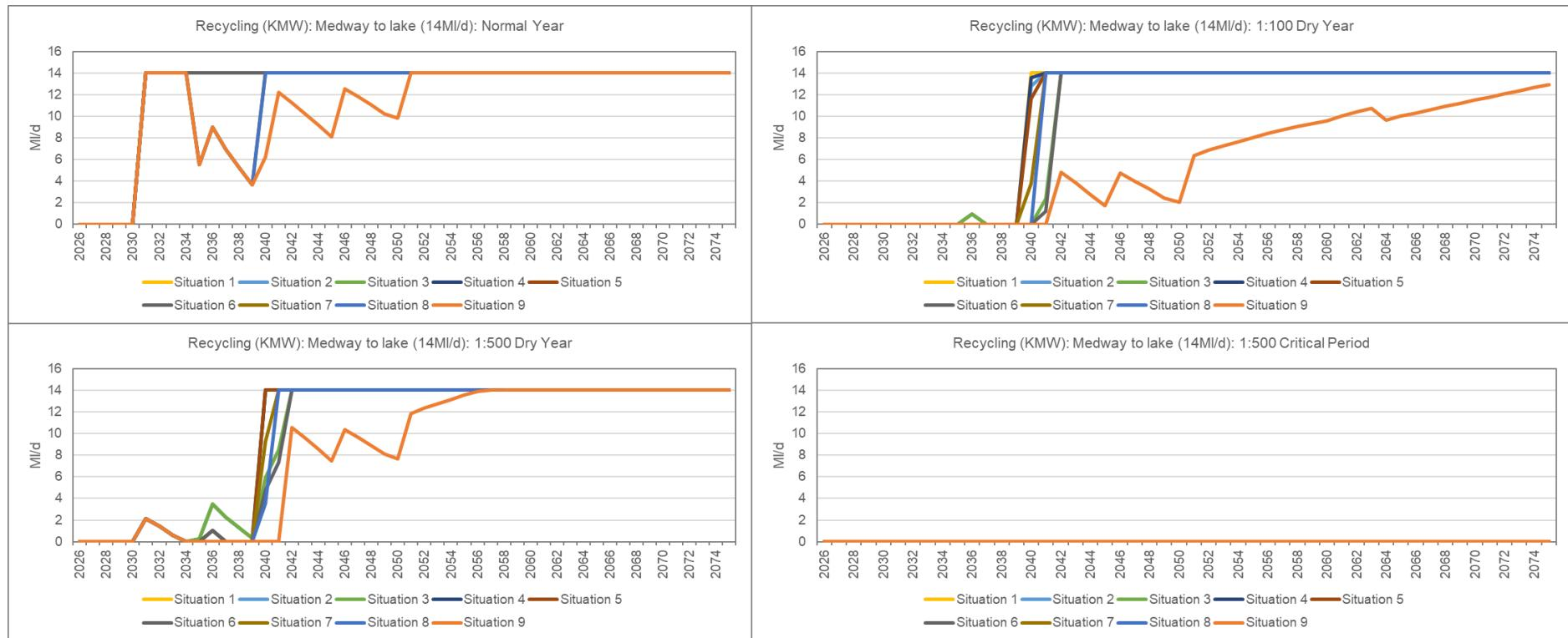
**Figure 68: Utilisation of Medway recycling option in KMW in each supply-demand situation under each planning scenario.**
