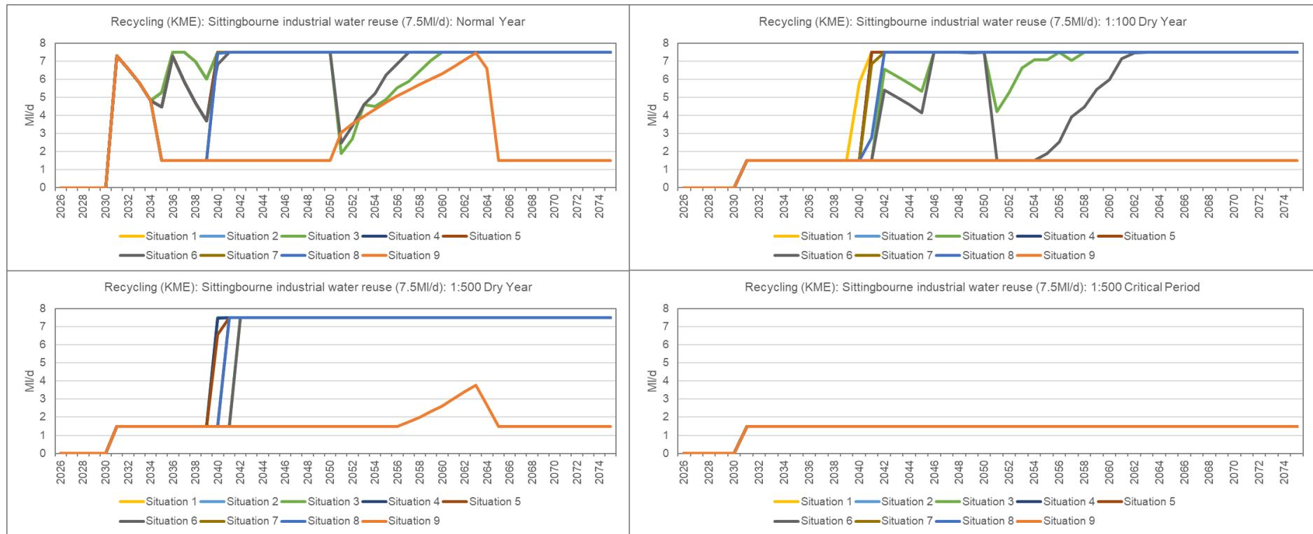
**Figure 67: Utilisation of Sittingbourne industrial water reuse option in KME in each supply-demand situation under each planning scenario.**
