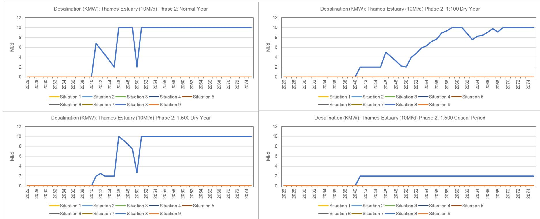
**Figure 59: Utilisation of Thames Estuary desalination option (10Ml/d Phase 2) in KMW in each supply-demand situation under each planning scenario.**
