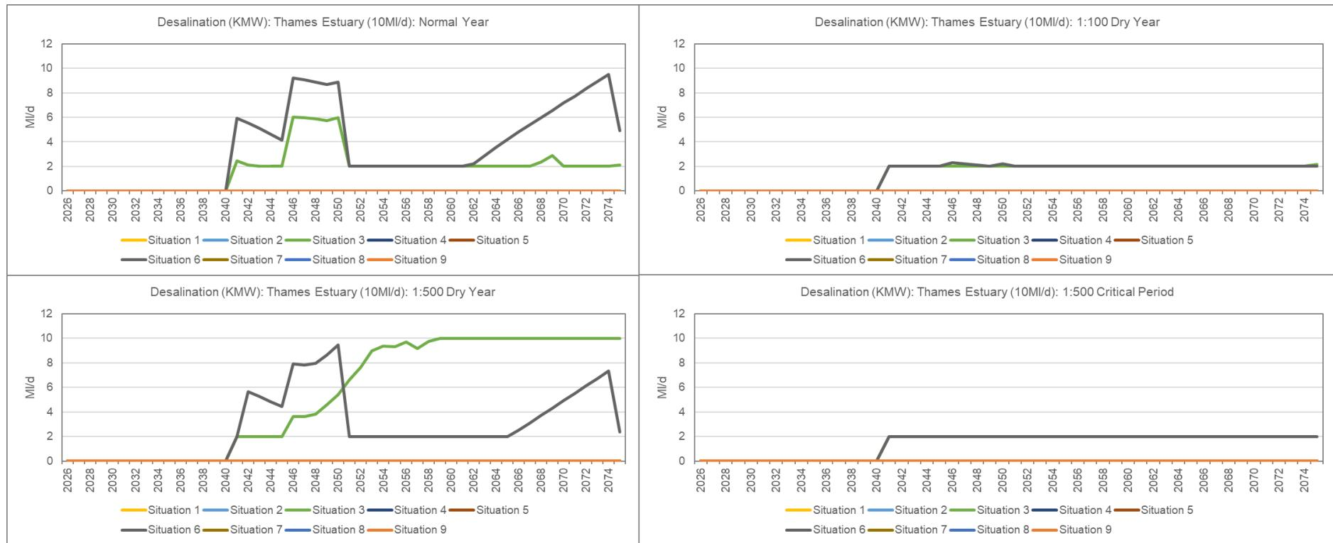
**Figure 58: Utilisation of Thames Estuary desalination option (10Ml/d) in KMW in each supply-demand situation under each planning scenario.**
