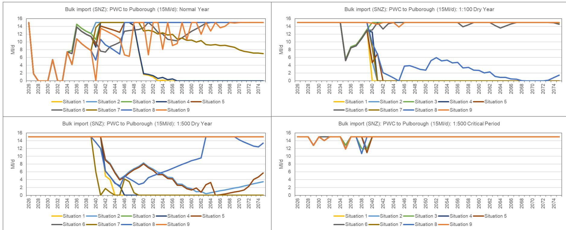
**Figure 27: Utilisation of bulk import from Portsmouth Water to Pulborough in SNZ in each supply-demand situation under each planning scenario.**
