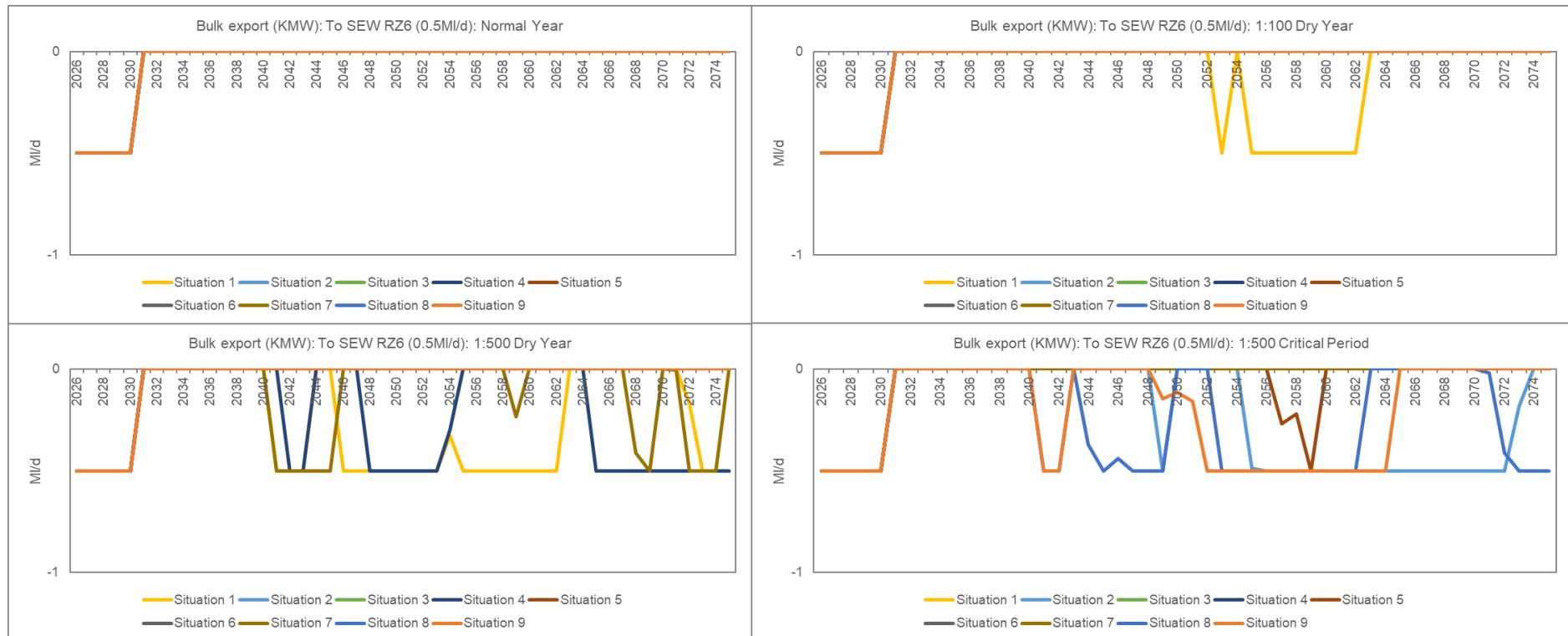
**Figure 46: Utilisation of bulk export from KMW to South East Water at Pitfield in each supply-demand situation under each planning scenario.**
