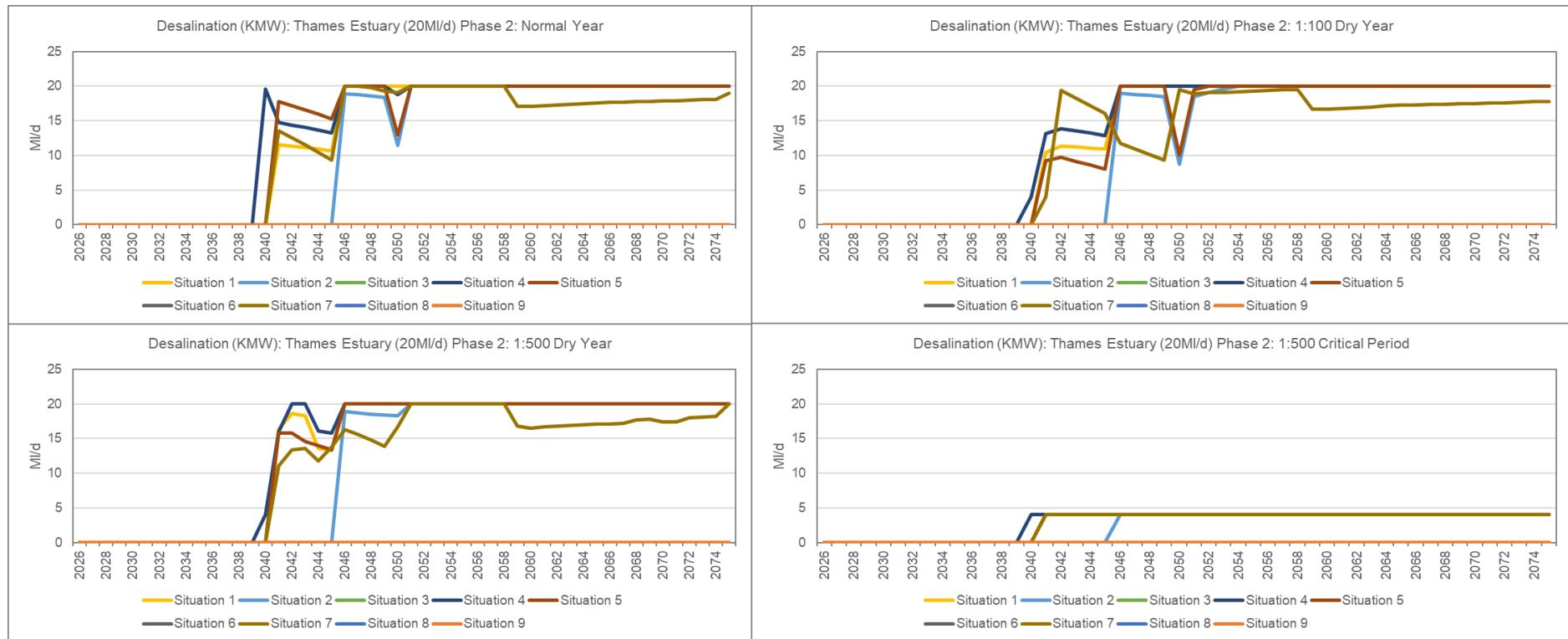
**Figure 61: Utilisation of Thames Estuary desalination option (20Ml/d Phase 2) in KMW in each supply-demand situation under each planning scenario.**
