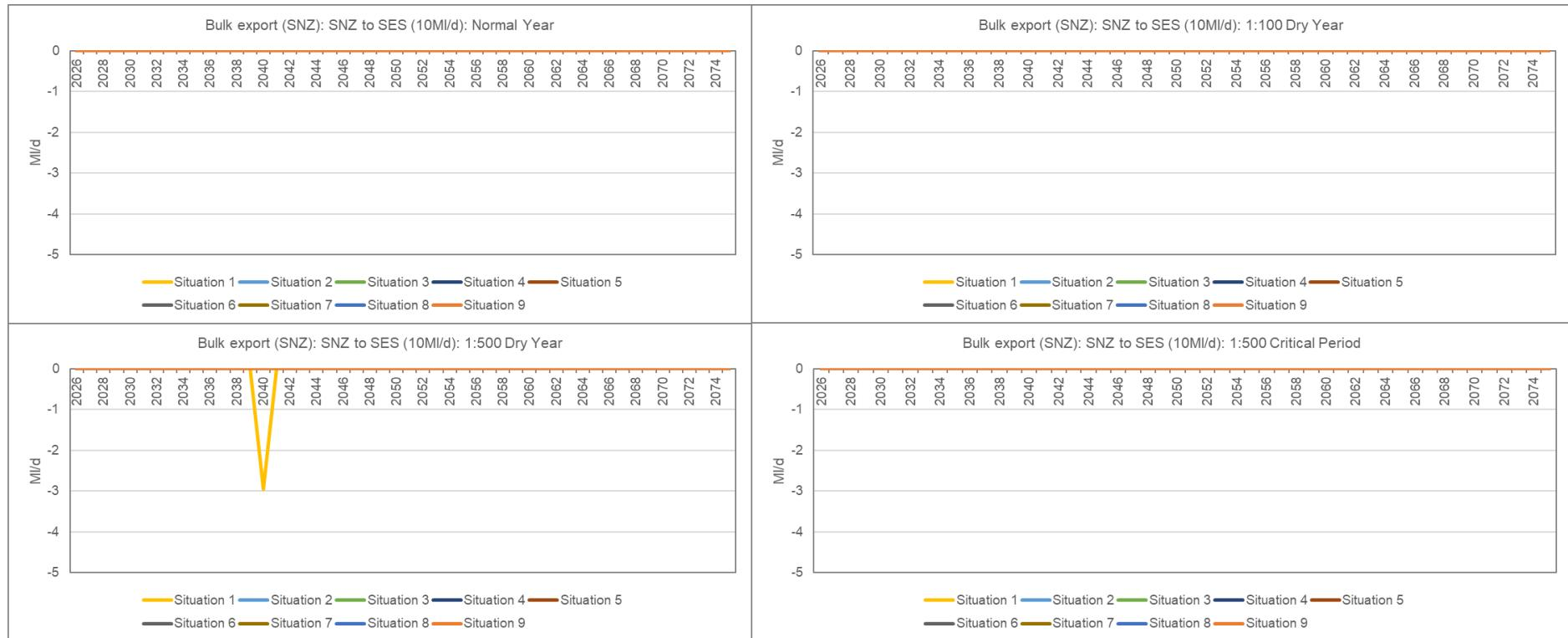
Figure 23: Utilisation of bulk export from SNZ to SES Water in each supply-demand situation under each planning scenario.
