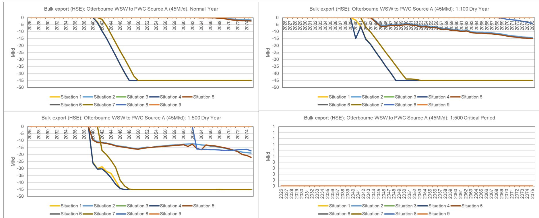
**Figure 1: Utilisation of bulk export from Otterbourne WSW HSE to Portsmouth Water Source A in each supply-demand situation under each planning scenario.**
