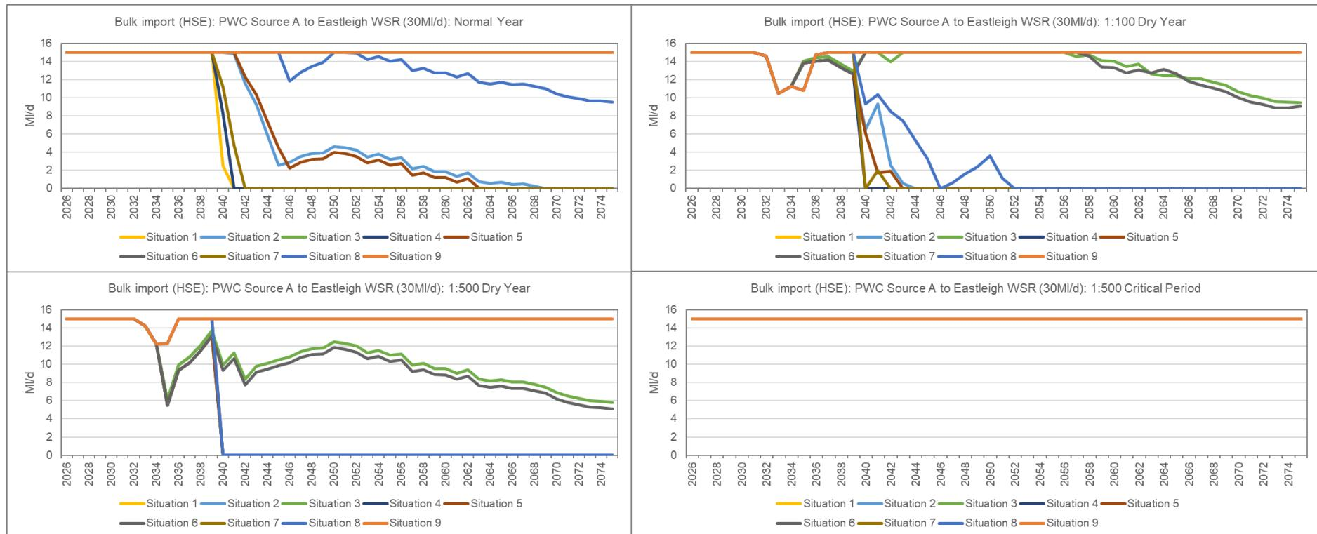
**Figure 6: Utilisation of bulk import to Eastleigh WSR in HSE from Portsmouth Water Source A in each supply-demand situation under each planning scenario.**
