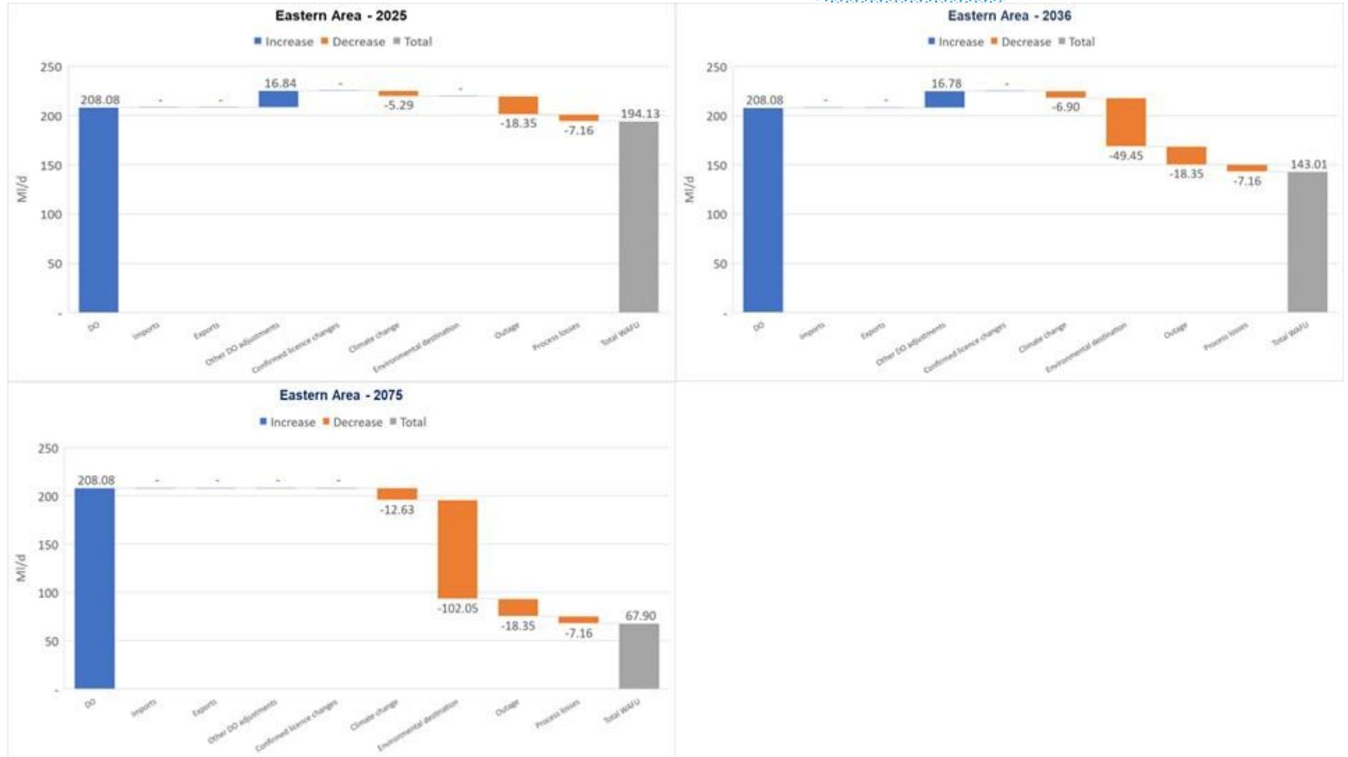
Figure 7.4: Forecast WAFU (MI/d) in the Eastern area under supply-demand Situation 4.
